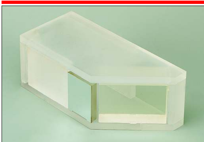
Figure 3. Representational view of the monolithic interferometer.
